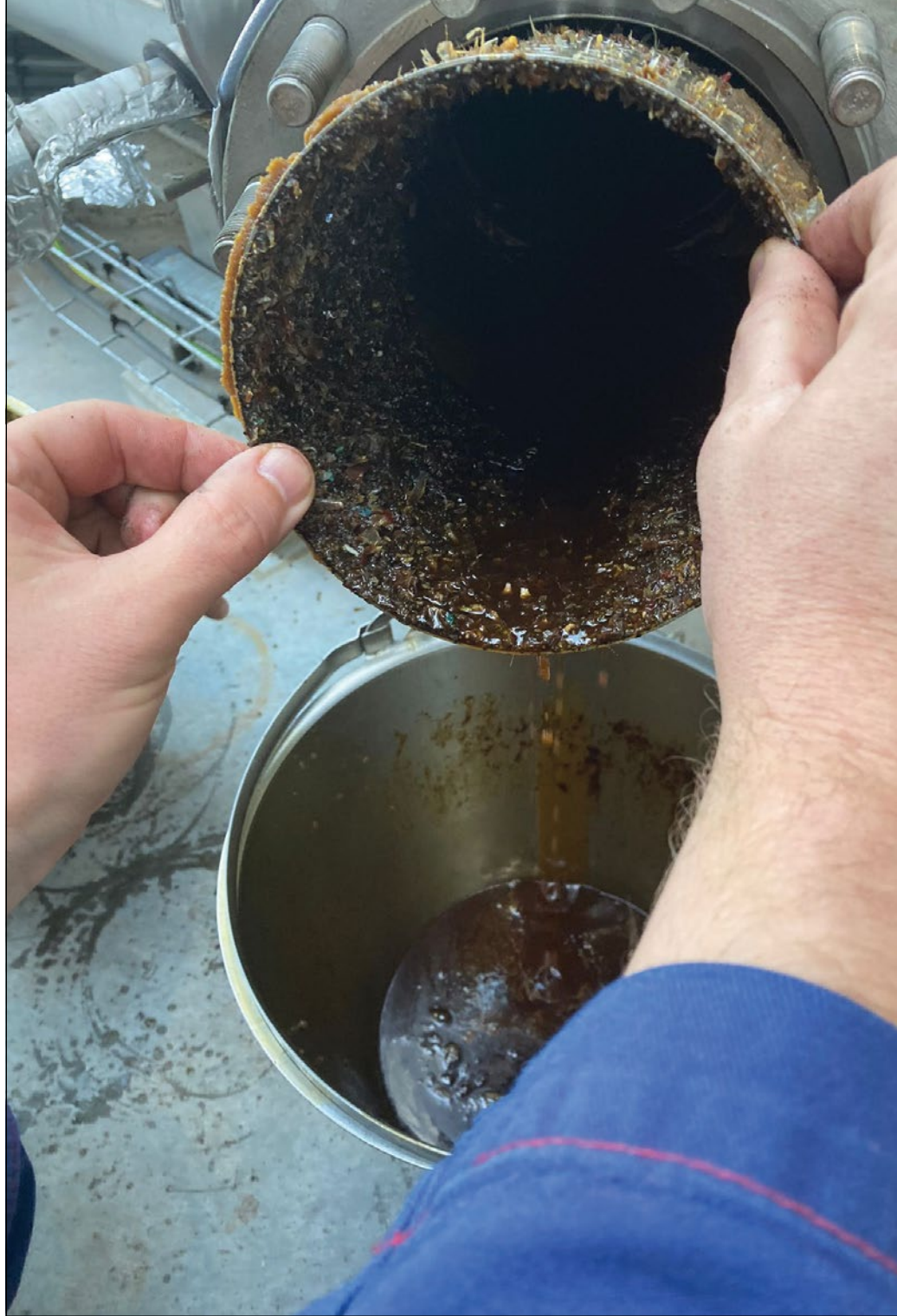
Polyethylene plastic in waste-based feedstock, such as that shown here in used cooking oil, can cause serious production issues if not removed in pretreatment.
